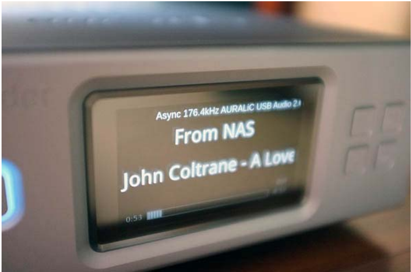
The Aurender handles DSD via DoP so the AMOLED readout reads "176.4" even though the file being sent is DSD
